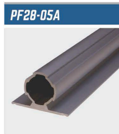
Material: A6063-T5 / Clear Anodize Mass: 0.68 kg./m. 6 MAX. LENGTH
